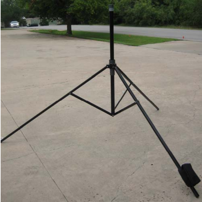
Picture of the Tripod fully extended. Notice by gripping and lifting on the center piece of the tripod, it helps to extend the legs with very little effort.
