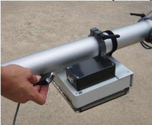
This picture illustrated the connection on the monitor assembly where you screw in the Control cable.
