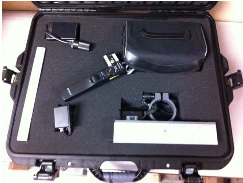
This is a Picture of the Contents of the RoverCam 23 Accessory case and contents. At the top left is the RoverCam 23 battery. Bottom Left is the RoverCam 23 Head assembly foot. To the Right of the Head foot assembly, is the RoverCam 23 Camera head monitor. In the middle is the RoverCam 23 control arm. In the Bottom Right is the RoverCam 23 Monitor assembly. At the top right is the camera bag.
