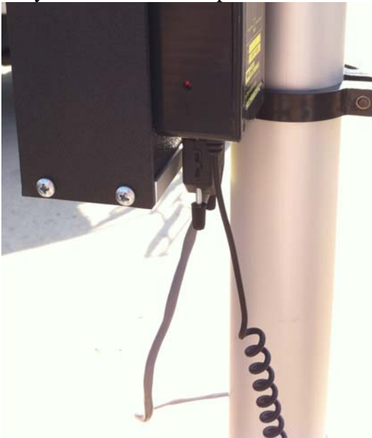
Picture of the molded end of the power cable that connects to the back of the monitor box.
