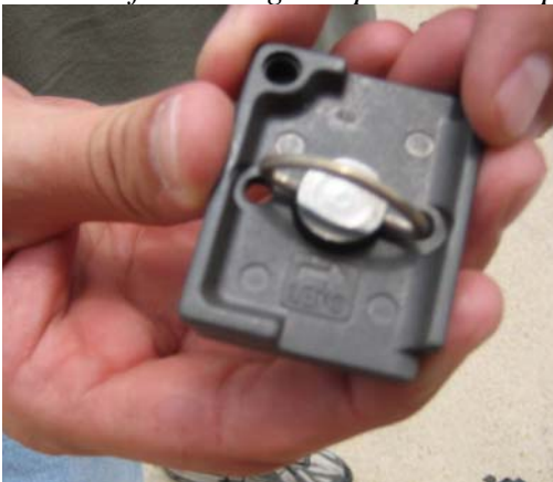
Picture of the quick release plate, once removed from the head assembly. Screw this onto the bottom of the camera, making sure that the diagram at the bottom reflects the way the camera lens is pointing.
