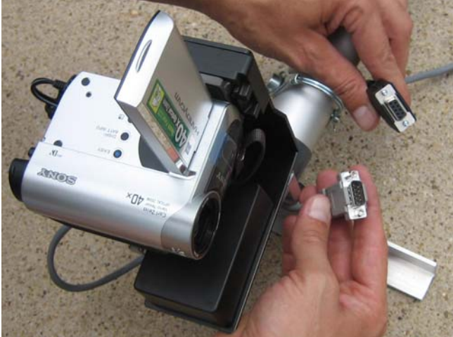
Connect the 9 pin Control cable connector
