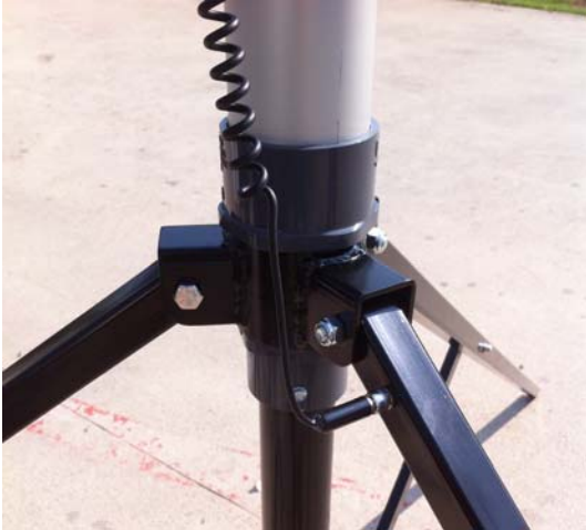
Picture of the Power Cable, that you would plug one end into the bottom of the Monitor assembly and the other end into the top of the tripods female power connection.
