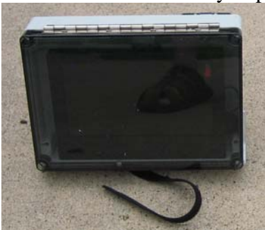
Picture of the Monitor Assembly before it has been clamped onto the RoverCam 23 mast.
