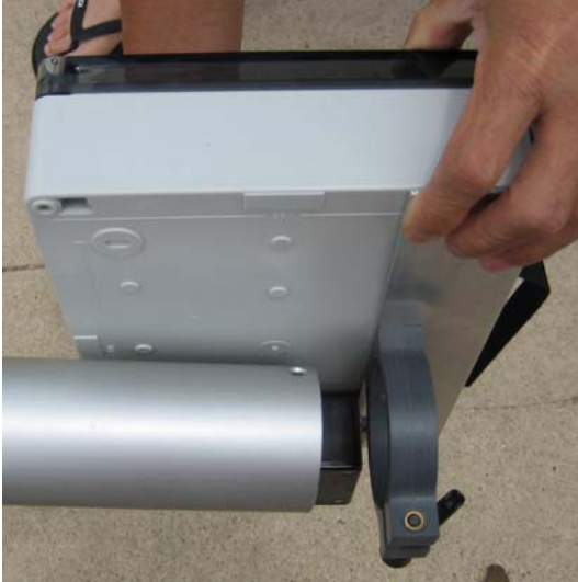
Picture of lining up the clamp for the RoverCam 23 on to the Bottom Mast section.
