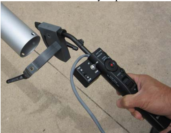
Picture of lining up the control arm at the bottom of the mast section to slide it up into place.
