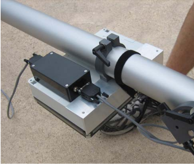
Picture of the Control arm cable plugged in and secured to the bottom of the monitor assembly.
