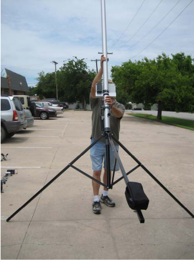
Picture of raising the RoverCam 23 by slowly walking the unit up. Slowly ease it up until the Tripod has all 3 legs firmly on the ground.
