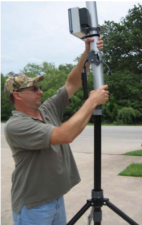
Picture of lifting the mast section and placing it over the tripod. Line up the holes and gently lower the mast section down into the tripod. It should fit fairly snug.
