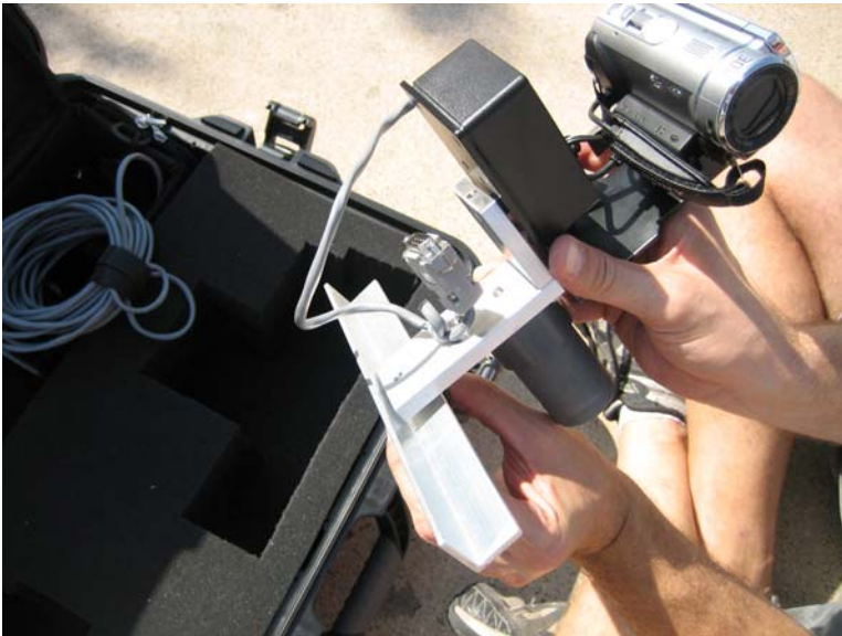
Shows picture of T-Rest plate being screwed in to the camera assembly.
