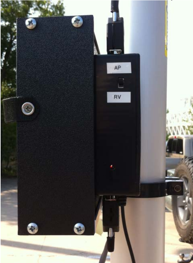
Picture of the Air Potato/RoverCam switch for those customers that have purchased the RoverCam 30 with the Air Potato
