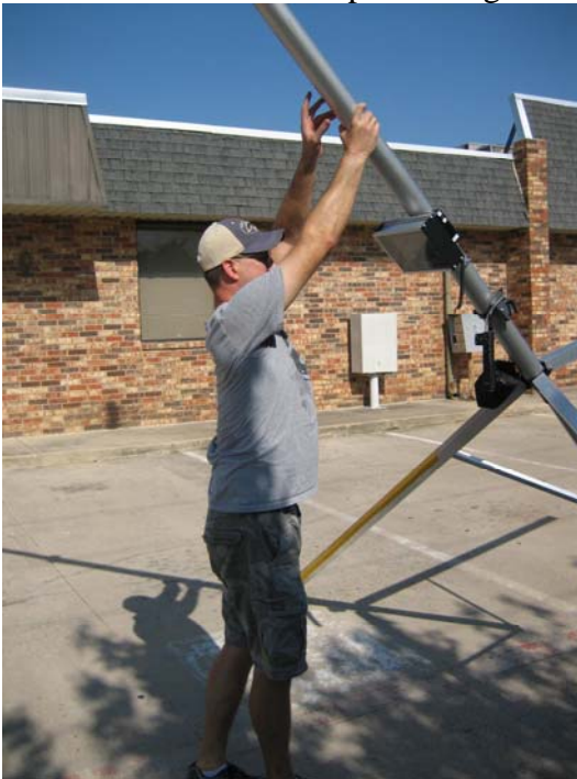
Picture of walking the mast section down to start telescoping the system.
