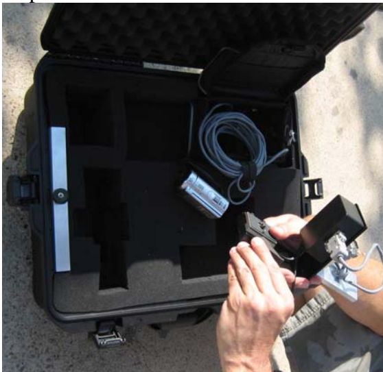
Picture of the Quick release plate before removal from the camera head assembly.
