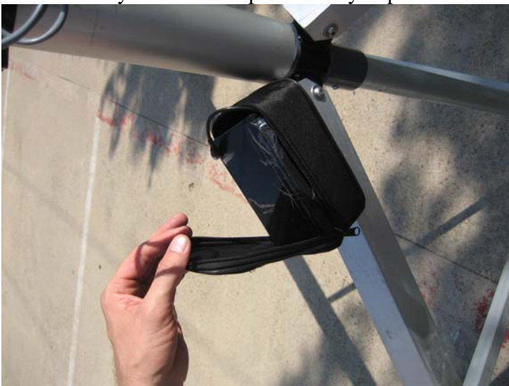
Picture of the battery before being zipped up into battery bag
