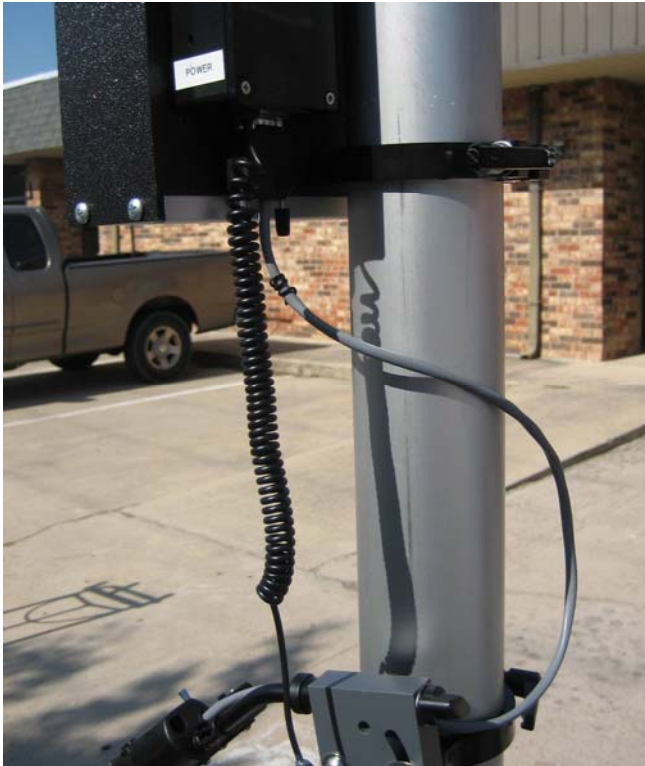
Picture of control arm screwed into bottom of monitor assembly
