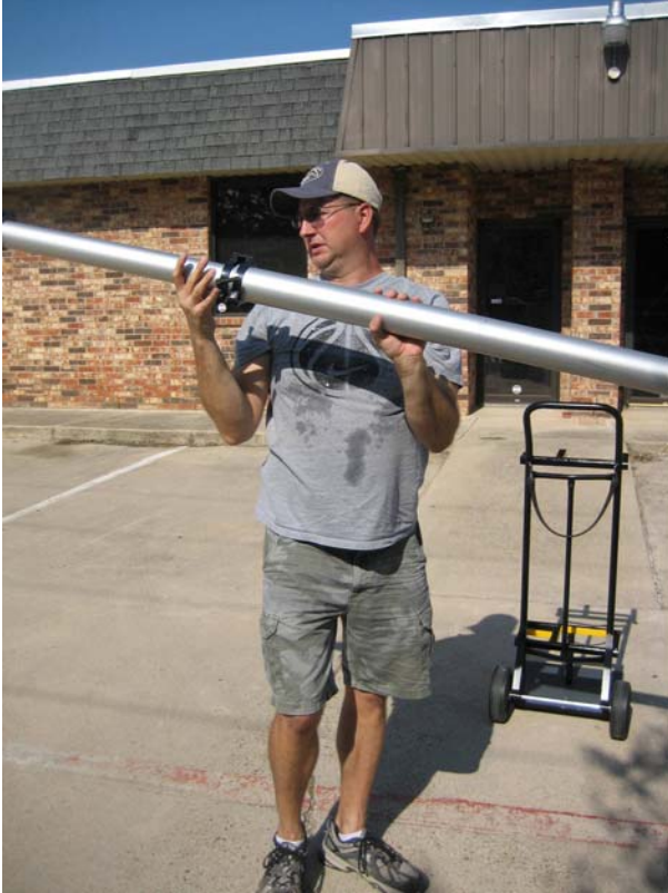
Picture of holding up the RoverCam 30 as you expand the lowest section of the mast. Twist the upper mast section clockwise to lock the mast section in place.
