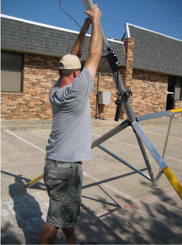
Picture of raising the RoverCam 30 by slowly walking the unit up. Slowly ease it up until the Tripod has all 3 legs firmly on the ground.
