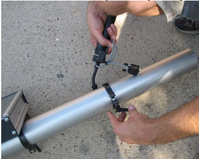
Picture of sliding the control assembly in place on the RoverCam 30 mast.
