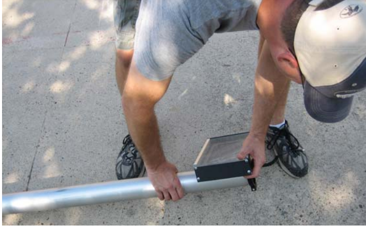
Picture of sliding the Monitor assembly onto the mast section of the RoverCam 30
