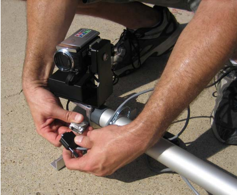
Connect the 9 pin Control cable connector
