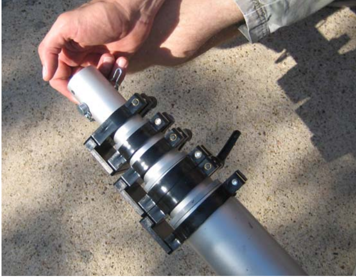
Picture of the Top of the Mast for the RoverCam 30. You would loosen the mast clamps by turning them on the handles at each clamp.
