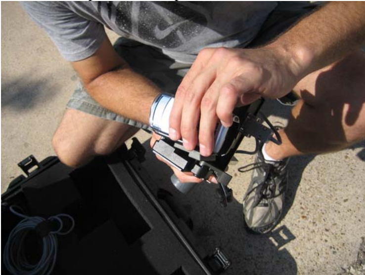
Picture of the Camera being locked into place once its attached to the quick release plate.
