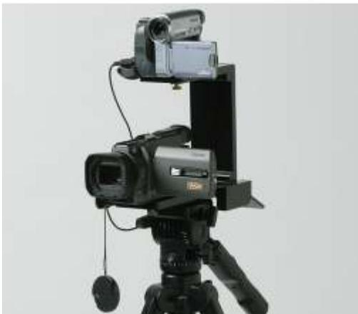
*Figure 1.3 Picture of 2 cameras mounted on a Dual Stack Bar*
