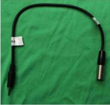
Figure 10.3 Picture of 2.5mm male to XLR female converter Cable for HIPOD EZ System
